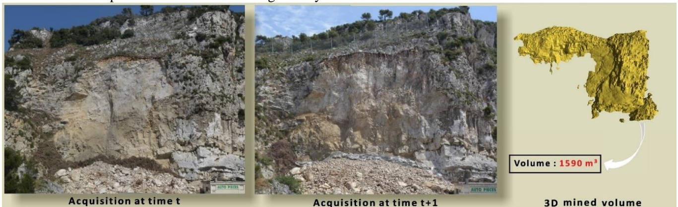
Figure 2 : The cliff before and after the blast + volume of mined rocks resulting from a laserscan of the cliff
